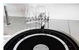
Washing Probe Independent 7-step washing system.
