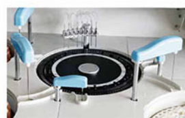
Reaction Tray 37±0.1°C, real-time monitor.
