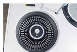
Reaction Tray 37±0.1°C, real-time monitor.
